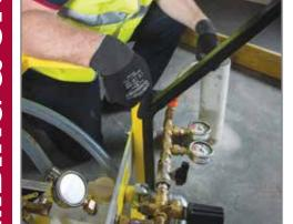
A manifold which can be hired out individually or with a pump for testing pressures between 1000 and 3000psi. Pump hose connects at one end and the other connects to the pipe. A built in unloader valve lets the operator to turn up the pressure during test.
