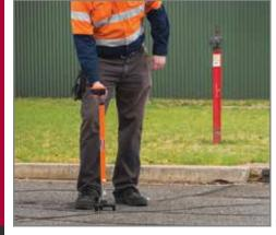
AquaTest T10 is a test rod used to electro acoustically locate leaks in water pipe networks. Water pipes being examined are picked up by the probe tip on the test rod can be detected as noise through the headphones.
